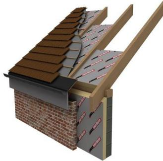
When insulating a pitched roof it is important to choose the right insulation type in order to reduce the risk of creating condensation, which can lead to mould and eventually damage to the building. Using IKO enertherm ALU insulation boards, with a moisture resistant cell structure, alongside an IKO Rubershield Breather Membrane (page 15) helps combat against condensation and reduce thermal bridging.
